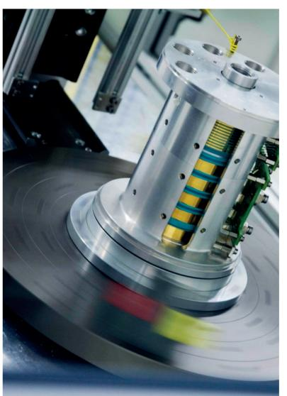
The slip ring is an essential device for the supply of power and the transmission of electrical signals. The quality of the slip ring is therefore a key factor for the quality of the overall system.
